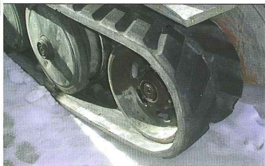
Figure 4. Pbv 302 fitted with a conventional rubber band-track from Good Year.
